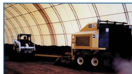
A Scat Turner breaks up, mixes and aerates the two compost windrow piles
