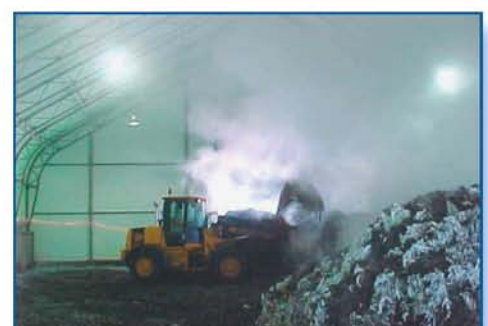
Machine operator forms stockpile into compost windrow.
